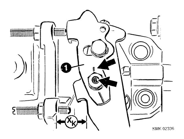
ADJUSTING CONTROL-LEVER POSITION "XK"
